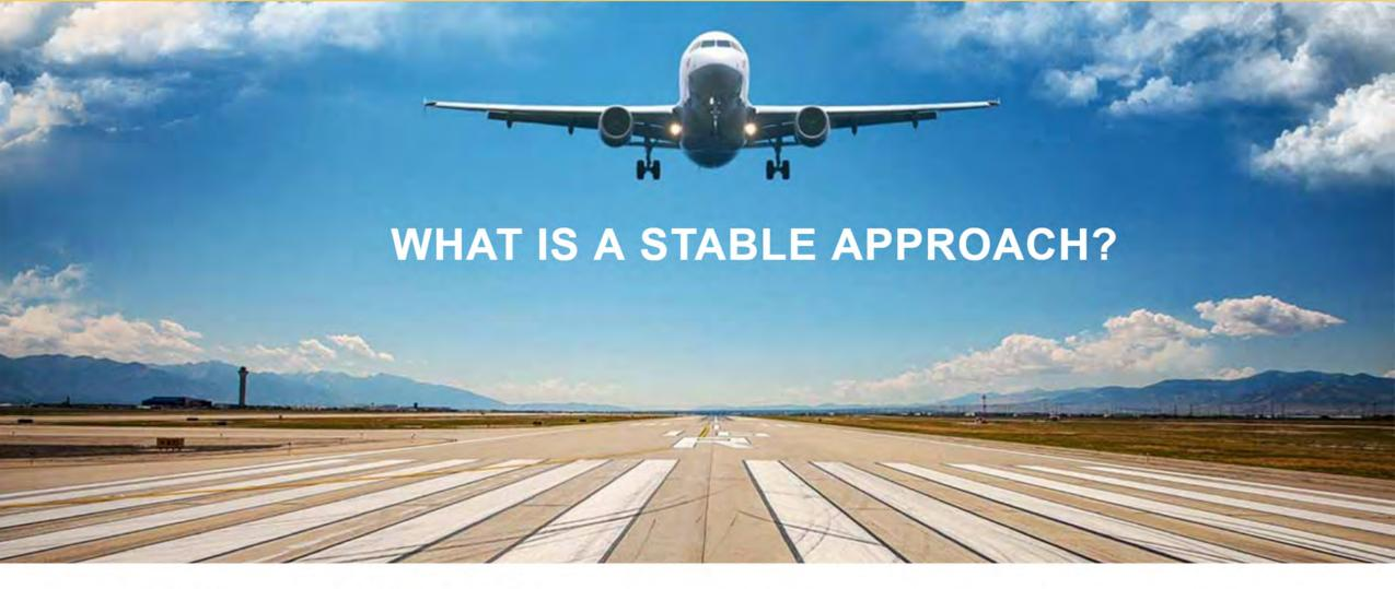
A stable approach is one in which the pilot establishes and maintains a constant angle glidepath towards a predetermined point on the landing runway. It is based on the pilot's judgment of certain visual clues and depends on the maintenance of a constant final descent airspeed and configuration.
